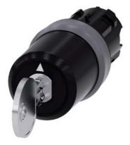
Key-operated switch BKS, 22 mm, round, plastic with metal front ring, lock number S1, with 2 keys, 3 switch positions I-O-II, latching, actuating angle  $2x45^{\circ}$ , 10:30h/12h/13:30h, Key removal I+II
