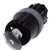
key-operated switch Siemens, 22 mm, round, plastic with metal front ring, lock number SSG10, with 2 keys, 2 switch positions O-I, latching, actuating angle 90°, 10:30h/13:30h, key removal O
