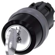
RONIS key-operated switch, 22 mm, round, plastic with metal front ring, lock number SB30, with 2 keys, 3 switch positions I-O<II, left latching, right momentary contact type, actuating angle 2x45°, 10:30h/12h/13:30h, key removal O+I, possible special locks: SB31, 421, 455
