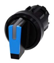
Selector switch, illuminable, 22 mm, round, plastic, blue, selector switch, short, 3 switch positions I>O<II, momentary contact type, actuating angle  $2x45^{\circ}$ , 10:30h/12h/13:30h
