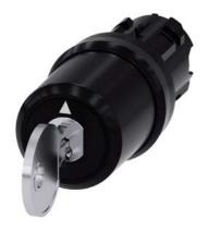
key-operated switch Siemens, 22 mm, round, plastic, lock number SSG10, with 2 keys, 3 switch positions I-O-II, latching, actuating angle 2x45°, 10:30h/12h/13:30h, key removal II
