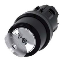
RONIS key-operated switch, 22 mm, round, plastic, lock number 455, with 2 keys, 2 switch positions O-I, latching, actuating angle  $90^\circ$ , 10:30h/13:30h, Key removal O+I
