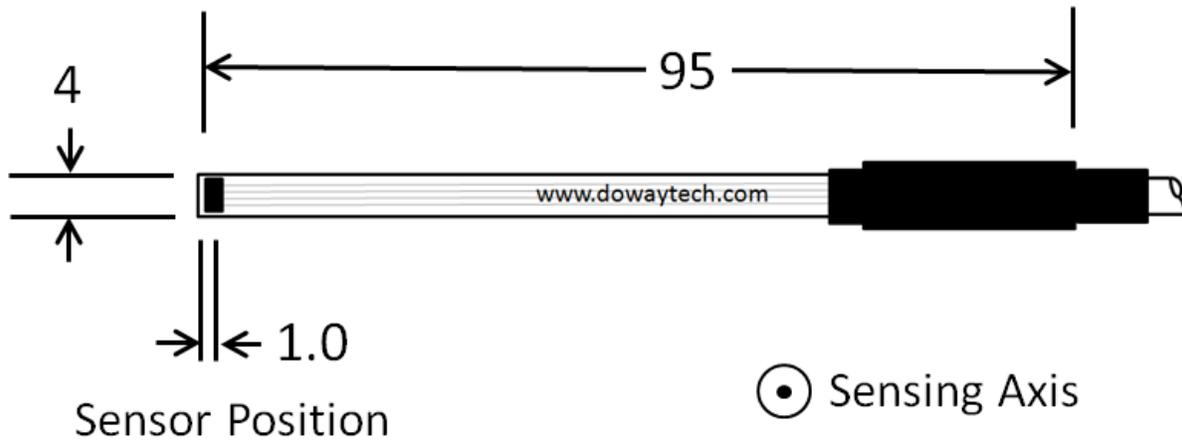
USB Connector and Rigid Probe view units: mm
