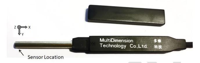
The USB magnetometer hardware is compatible with the popular open source Arduino UNO board, and thus with the Arduino programming environment or Atmel microcontroller development tools. The user may develop custom firmware at his/her risk. The hardware includes a boot loader for uploading Arduino code. The USB magnetometer hardware model is defined as follows:
