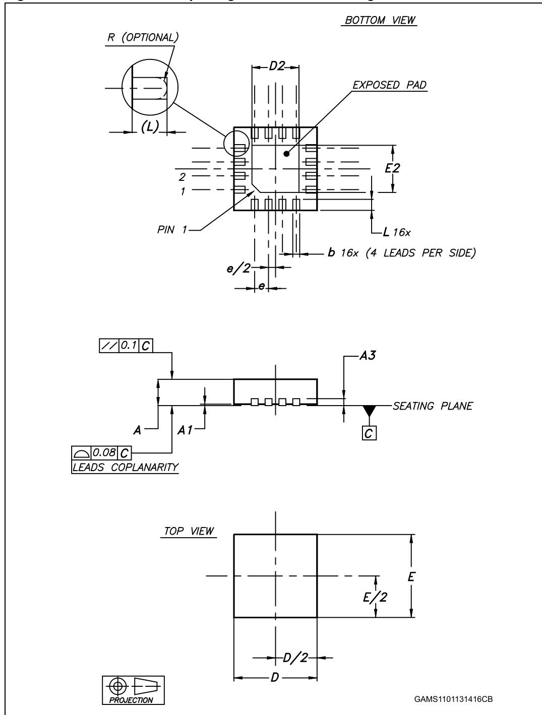
**Table 13.** QFN16 3 x 3 mm package mechanical data (pitch 0.5 mm)
