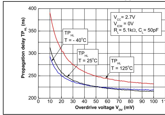
**Figure 19. Propagation delay versus overdrive with positive transition,  $V_{CC} = 2.7V$**
