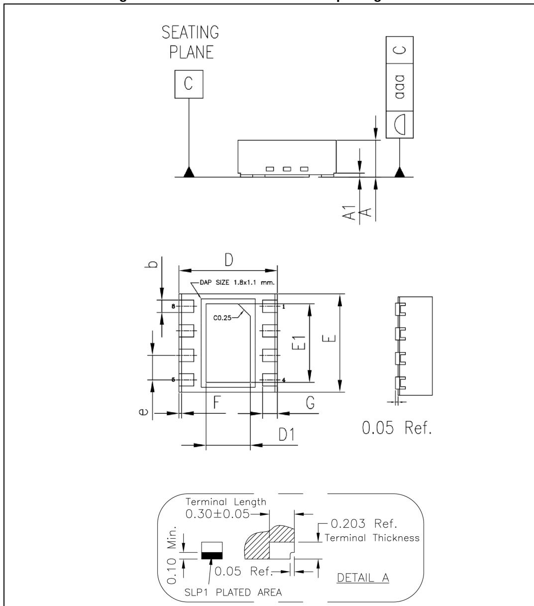
**Table 10.** DFN8 2 x 2 wettable flank package mechanical data
