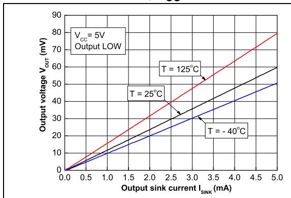
**Figure 13. Output sink current versus output voltage**
