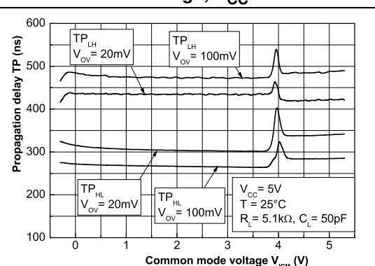
**Figure 24. Propagation delay versus time with negative transition**
