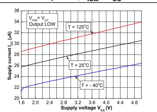
**Figure 6. Supply current versus temperature**
