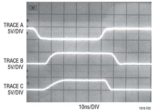
Figure 2. LT1016 vs a TTL Gate
