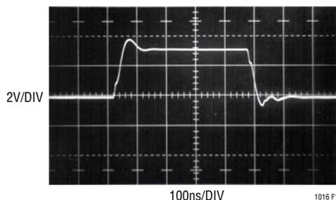
**Figure 12. Excessive Load Capacitance Forces Edge Distortion**
