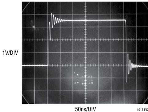
**Figure 13. Lengthy, Unterminated Output Lines Ring from Reflections**
