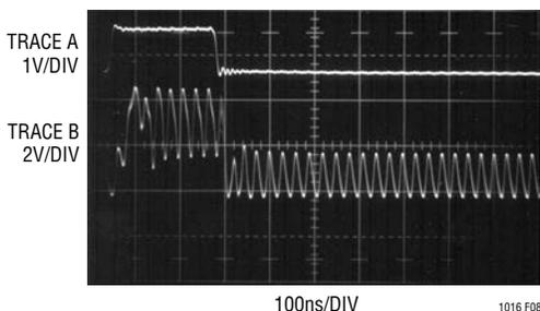
Figure 8. Excessive LT1016 Ground Path Resistance Causes Oscillation
