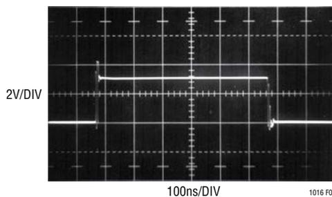
Figure 9. Transition Instabilities Due to No Ground Plane
