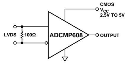
Figure 13. LVDS-to-CMOS Receiver
