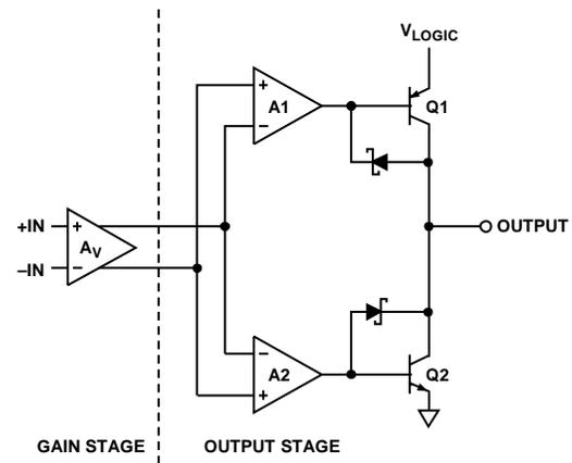
Figure 9. Simplified Schematic Diagram of TTL-/CMOS-Compatible Output Stage
