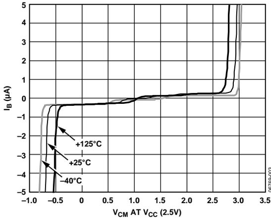
Figure 3. Input Bias Current vs. Input Common-Mode Voltage
