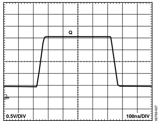
Figure 7. 1 MHz Output Voltage Waveform  $V_{CC} = 2.5\text{ V}$
