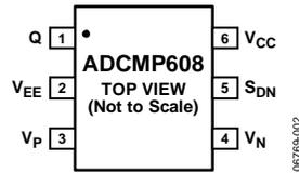
Figure 2. Pin Configuration
