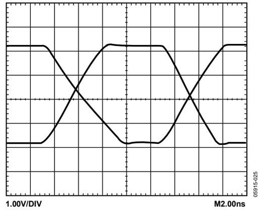
Figure 13. 50 MHz Output Voltage Waveform at  $V_{CCO} = 5.5 V$
