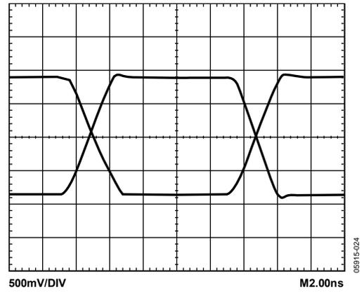
Figure 12. 50 MHz Output Voltage Waveform at  $V_{CCO} = 2.5 V$
