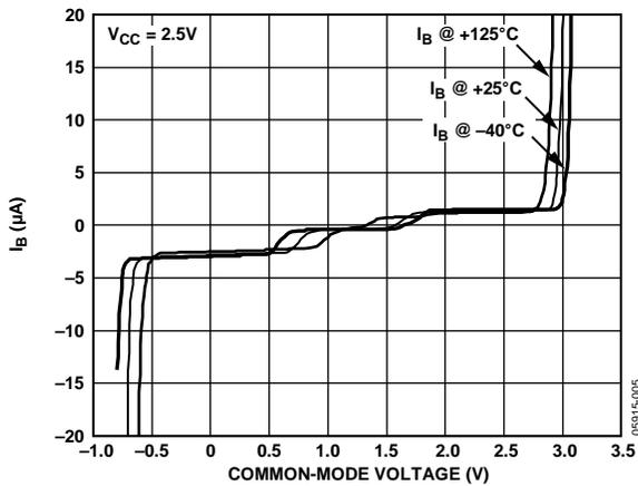
Figure 6. Input Bias Current vs. Input Common Mode
