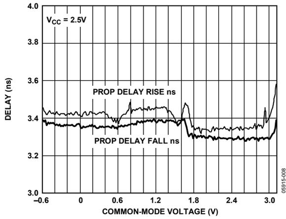
Figure 11. Propagation Delay vs. Input Common Mode
