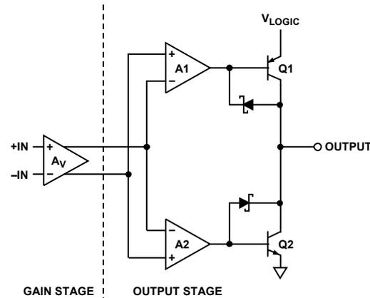
Figure 14. Simplified Schematic Diagram of TTL-/CMOS-Compatible Output Stage
