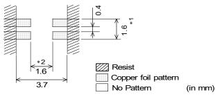
\*1 If the pattern is made with wider than 1.6mm. It will result to let component turn around, because melting speed is different. In the worst case, short circuit between lines may be occured.
