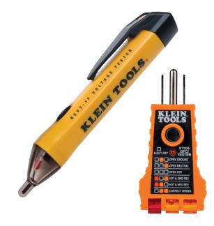
Klein Tools Test Kit includes the NCVT1P Non-Contact Voltage Tester and RT205 GFCI Receptacle Tester. The Non-Contact Voltage Tester detects standard voltage in cables, cords, circuit breakers, lighting fixtures, switches, non tamper-resistant outlets and wires. The GFCI Receptacle Tester detects the most common wiring problems in standard receptacles.
