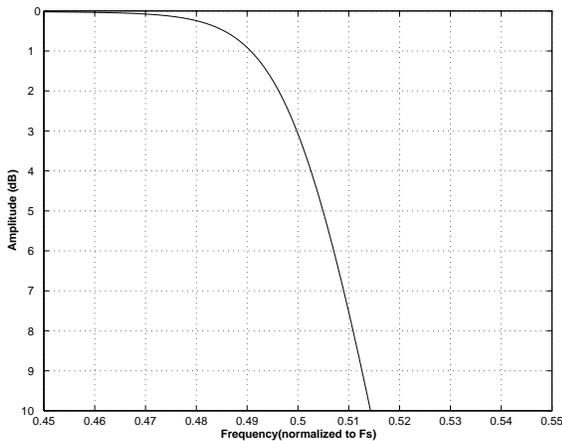
**Figure 31. DAC Double Speed (fast) Transition Band (detail)**
