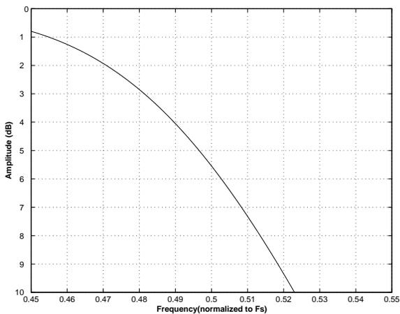
**Figure 43. DAC Quad Speed (slow) Transition Band (detail)**
