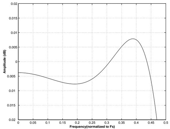
**Figure 24. DAC Single Speed (fast) Passband Ripple**
