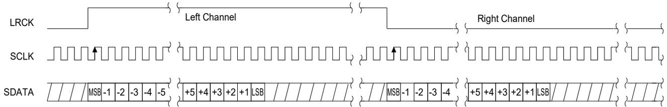
**Figure 3. Format 0, Left Justified up to 24-Bit Data**
