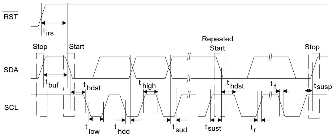
Figure 6. I<sup>2</sup>C Mode Control Port Timing
