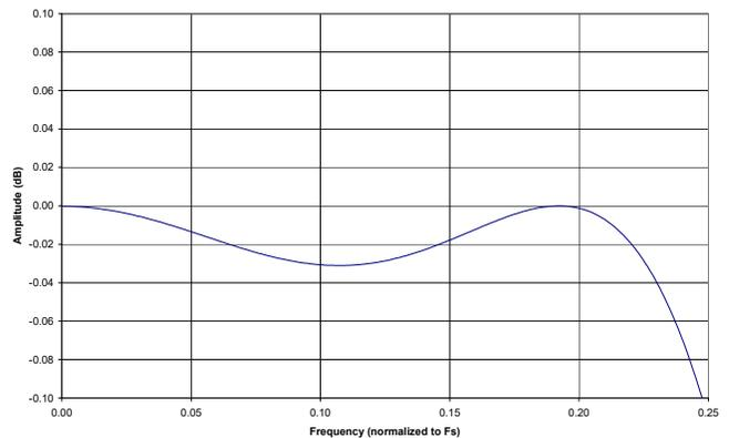
**Figure 56. ADC Quad Speed Mode Passband Ripple**
