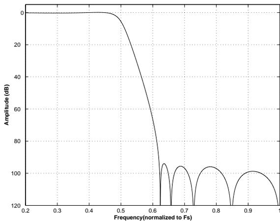
**Figure 37. DAC Quad Speed (fast) Stopband Rejection**
