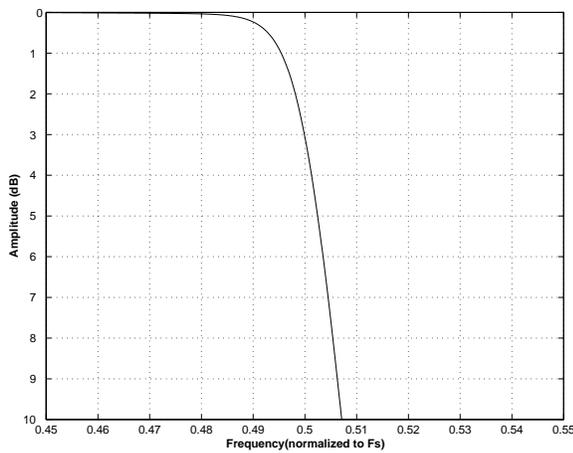
**Figure 23. DAC Single Speed (fast) Transition Band (detail)**
