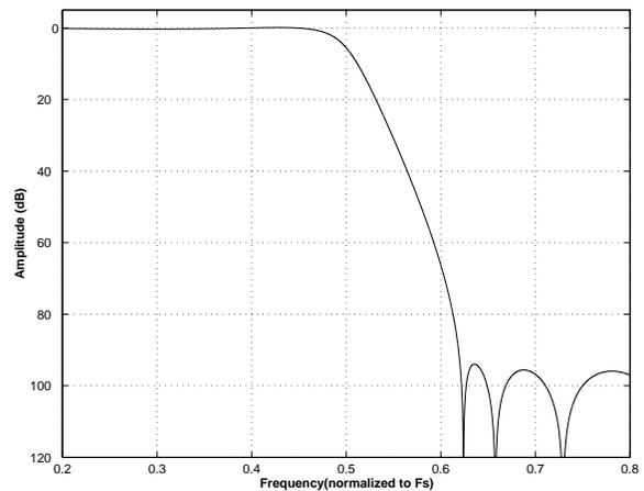
**Figure 38. DAC Quad Speed (fast) Transition Band**
