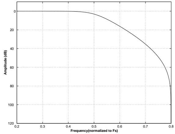
**Figure 34. DAC Double Speed (slow) Transition Band**
