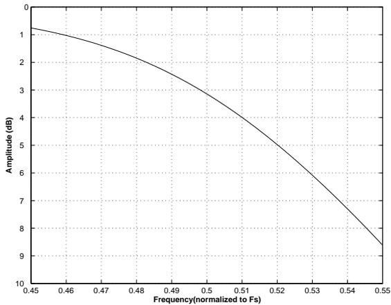
**Figure 35. DAC Double Speed (slow) Transition Band (detail)**
