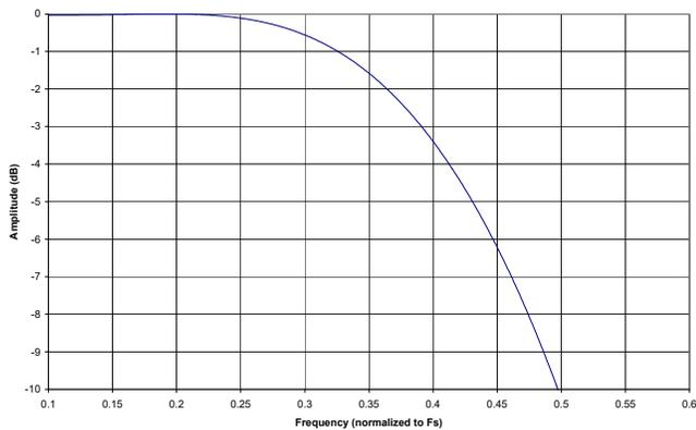
**Figure 55. ADC Quad Speed Mode Transition Band (Detail)**
