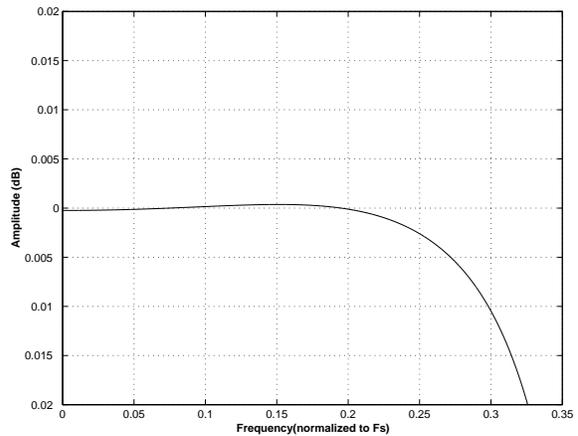
**Figure 36. DAC Double Speed (slow) Passband Ripple**
