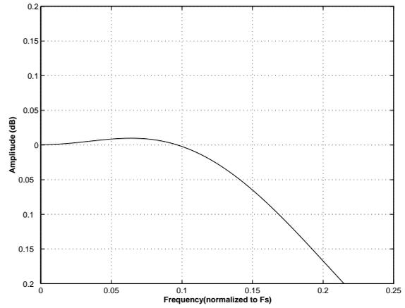
**Figure 40. DAC Quad Speed (fast) Passband Ripple**
