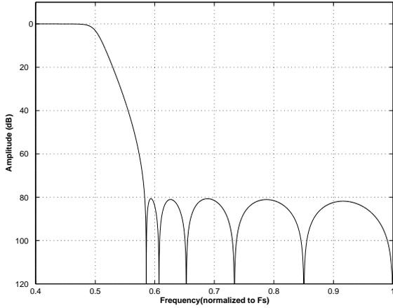
**Figure 29. DAC Double Speed (fast) Stopband Rejection**
