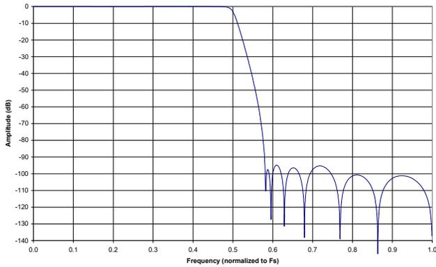
**Figure 45. ADC Single Speed Mode Stopband Rejection**
