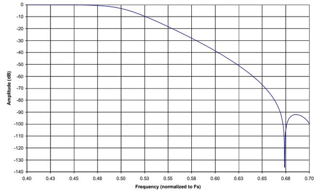
**Figure 50. ADC Double Speed Mode Transition Band**
