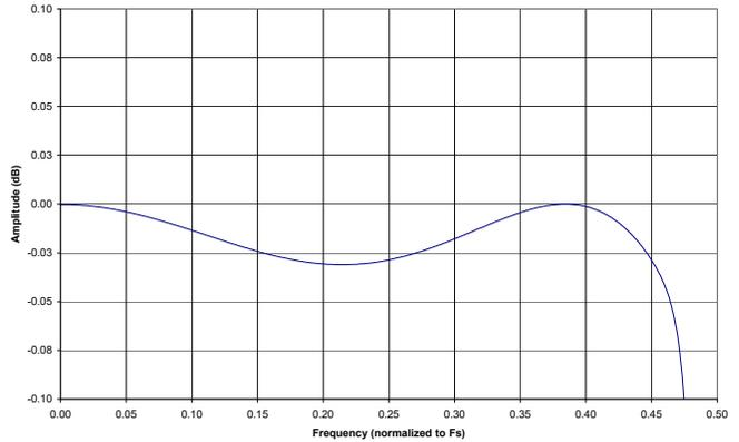
**Figure 48. ADC Single Speed Mode Passband Ripple**
