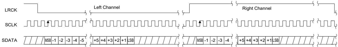
**Figure 4. Format 1, I²S up to 24-Bit Data**
