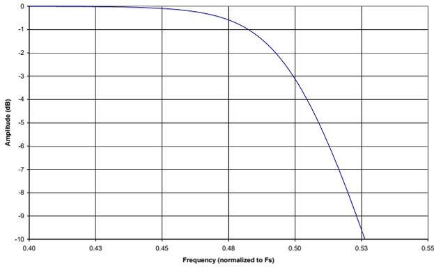
**Figure 51. ADC Double Speed Mode Transition Band (Detail)**
