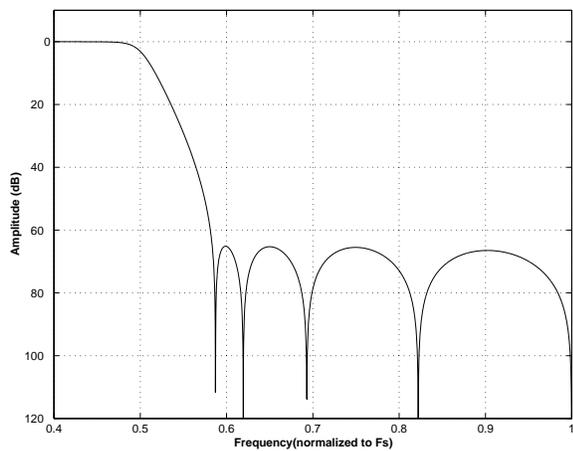
**Figure 25. DAC Single Speed (slow) Stopband Rejection**
