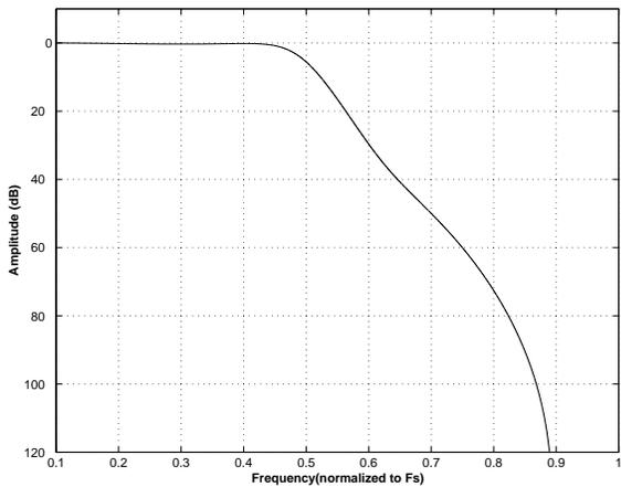
**Figure 41. DAC Quad Speed (slow) Stopband Rejection**
