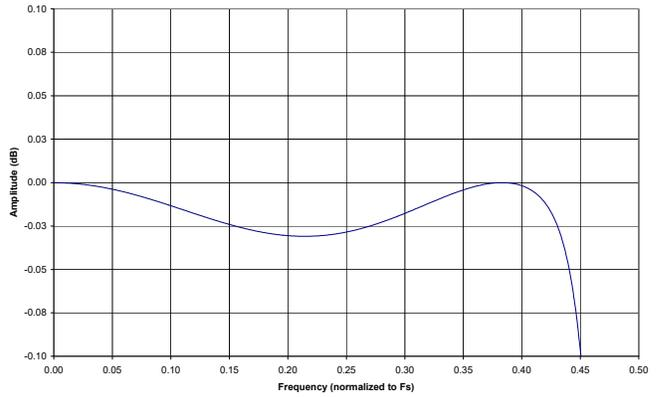
**Figure 52. ADC Double Speed Mode Passband Ripple**
