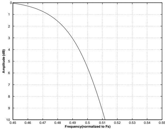
**Figure 39. DAC Quad Speed (fast) Transition Band (detail)**
