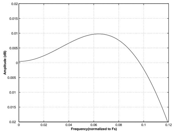
**Figure 44. DAC Quad Speed (slow) Passband Ripple**
