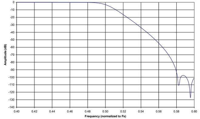
**Figure 46. ADC Single Speed Mode Transition Band**
