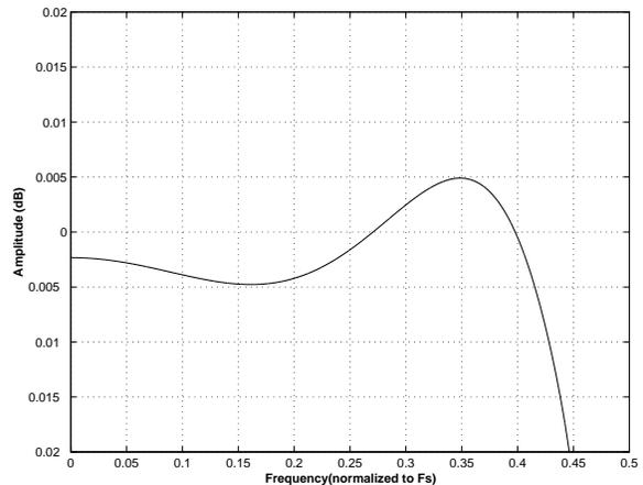
**Figure 32. DAC Double Speed (fast) Passband Ripple**
