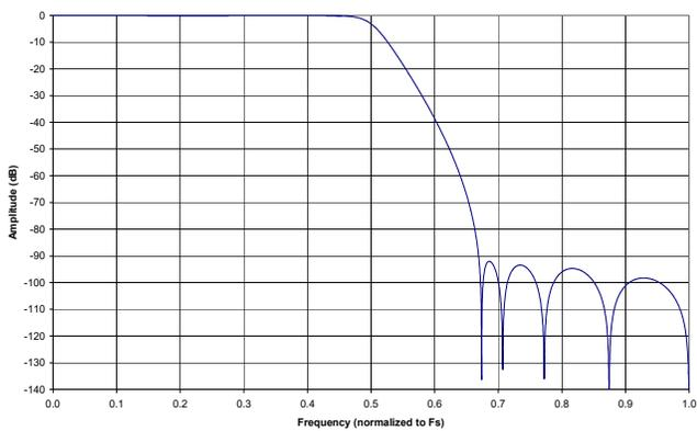
**Figure 49. ADC Double Speed Mode Stopband Rejection**
