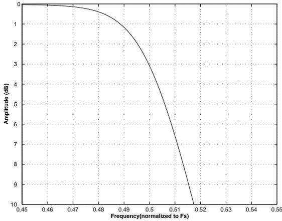
**Figure 27. DAC Single Speed (slow) Transition Band (detail)**
