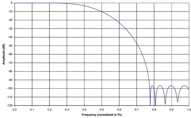
**Figure 53. ADC Quad Speed Mode Stopband Rejection**
