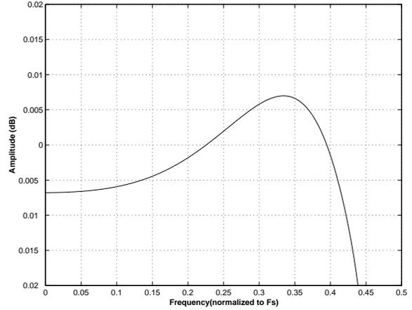
**Figure 28. DAC Single Speed (slow) Passband Ripple**
