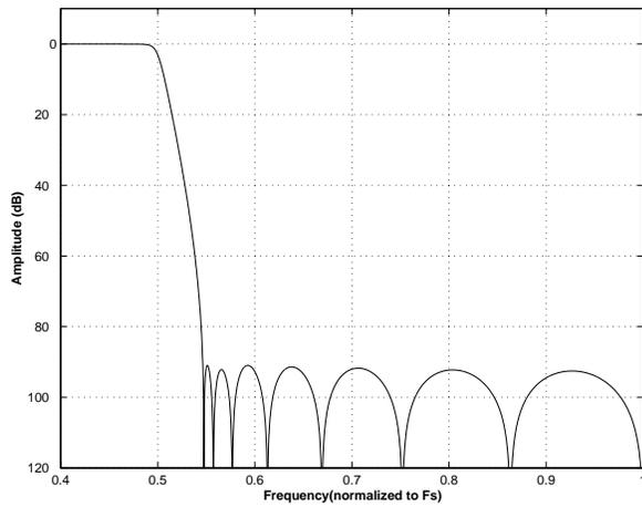
**Figure 21. DAC Single Speed (fast) Stopband Rejection**
