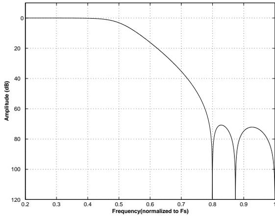
**Figure 33. DAC Double Speed (slow) Stopband Rejection**
