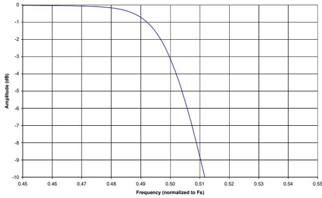
**Figure 47. ADC Single Speed Mode Transition Band (Detail)**
