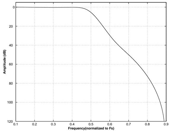
**Figure 42. DAC Quad Speed (slow) Transition Band**
