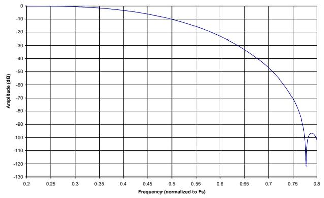
**Figure 54. ADC Quad Speed Mode Transition Band**
