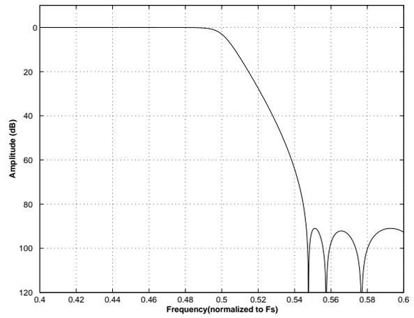
**Figure 22. DAC Single Speed (fast) Transition Band**
