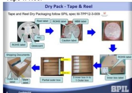
**Note:** Tray vendor (Hwa Shu) and Tape-n-Reel vendor (Advantek) are qualified suppliers for Cirrus Logic. All BEOL (Back End Of Line) processing adheres to Cirrus Logic established standards.
