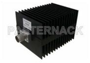
High Power 100 Watts RF Load Up To 4 GHz With N Male Input Square Body Black Anodized Aluminum Heatsink
