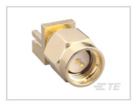
RF Interface: SMA RF Connector Style: Plug Impedance: 50 Ω RF Connector Coupling Mechanism: Threaded Operating Frequency: 0–18 GHz
