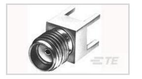
RF Interface: SMA RF Connector Style: Jack RF Connector Mated Outer Diameter (Approximate): 8.99 mm [.354 in] Impedance: 50 Ω RF Connector Coupling Mechanism: Threaded
