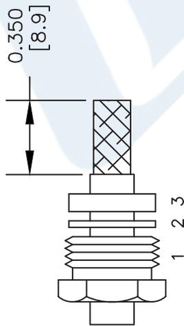
FORM BRAID OVER CLAMP NUT (4). TRIM BRAID BACK TO SHOULDER. CUT DIELECTRIC & CENTER CONDUCTOR TO DIMENSION SHOWN. DO NOT NICK CENTER CONDUCTOR. SOLDER CONTACT TO CENTER CONDUCTOR. REMOVE EXCESS SOLDER. DO NOT OVER HEAT DIELECTRIC. INSERT CABLE ASSEMBLY INTO BODY & TIGHTEN.
