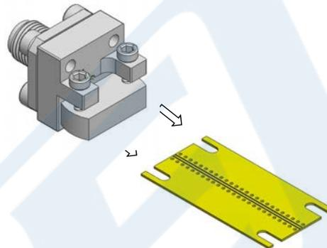
Step 3: Verify that the transition block is secured on the board.
