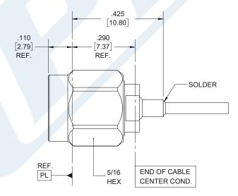
Click the following link (or enter part number in "SEARCH" on website) to obtain additional part information including price, inventory and certifications: 2.92mm Male Connector Solder Attachment for PECX001, PECX002, Low Loss 047 Semi-Rigid PE45483
