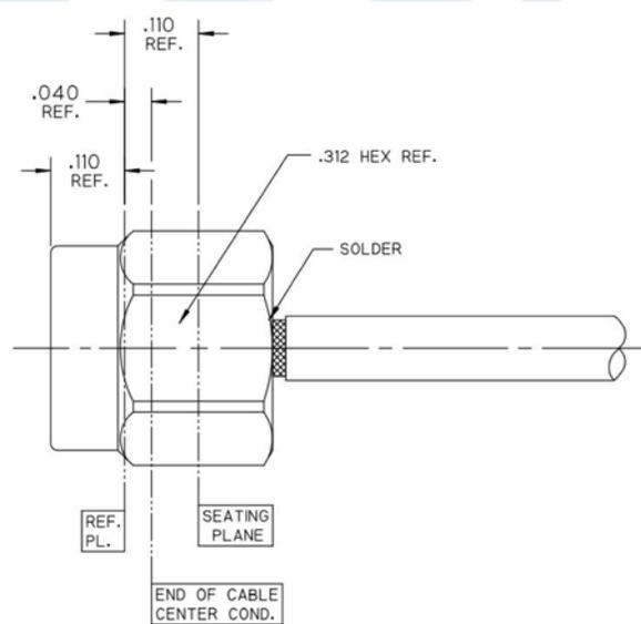
Click the following link (or enter part number in "SEARCH" on website) to obtain additional part information including price, inventory and certifications: [SMA Male Connector Solder Attachment for RG405, RG405 Tinned, PE-SR405AL, PE-SR-405FL, PE-SR405FLJ, PE-SR405TN PE45480](#)
