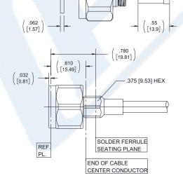
4. INSERT CABLE/CONTACT SUB-ASSEMBLY INTO THE CONNECTOR UNTIL SEATED. TIGHEN CONNECTOR COUPLING NUT TO MATING TYPE N JACK. TIGHTEN REAR CLAMP NUT TO 30-40 IN-LBS AND DISENGAGE MAIN INTERFACE FROM JACK.
