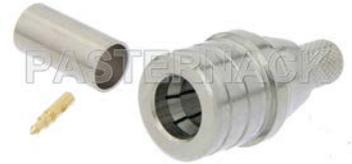
QMA Male Connector Crimp/Solder Attachment for PE-C195, PE-P195, RG58, RG141, RG303, LMR-195, 0.195 inch
