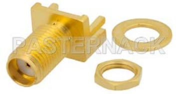
SMA Female Bulkhead Mount Connector Solder Attachment .042 inch End Launch PCB, .250 inch Diameter, .020 inch x .010 inch Contact
