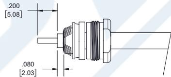
3. SLIDE WASHER (4) AGAINST THE BRAID CLAMP (3) AND HOLD BRAID IN PLACE. SLIDE HALF-INSULATOR (5) BEFORE SOLDER CONTACT (6) TO CENTER CONDUCTOR. SOLDER & REMOVE EXCESS SOLDER. DO NOT OVER HEAT DIELECTRIC. SLIDE A REST HAFT-INSULATOR (5) TO LOCKED CONTACT. INSERT CABLE ASSEMBLY INTO BODY (7) & TIGHTEN.
