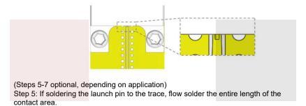
Step 6: To avoid performance mistakes, remove excess solder.
