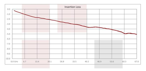
Measurement is for two connectors with 1.0 inch (25.4mm) length of substrate
