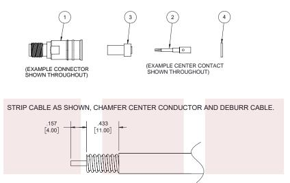
2. SLIDE THICKER INSULATOR ③ OVER CENTER CONTACT AND SLIDE THINNER INSULATOR ④ OVER CABLE CENTER CONDUCTOR. INSERT CENTER CONTACT AND SOLDER. WRAP THE CABLE BY SOLDER WIRE.
