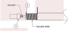
3. PUSH THE CONNECTOR BODY INTO THE CABLE, UNTIL IT STOPS. SOLDER THE CONNECTOR BODY WITH CABLE AND COVER HEATSHRINK SLEEVE.
