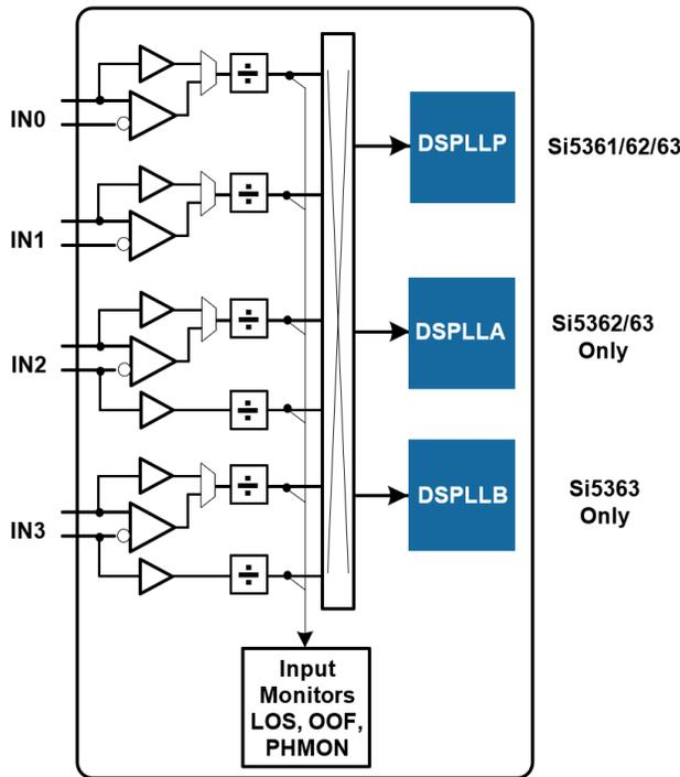
Figure 17. Input Structure
