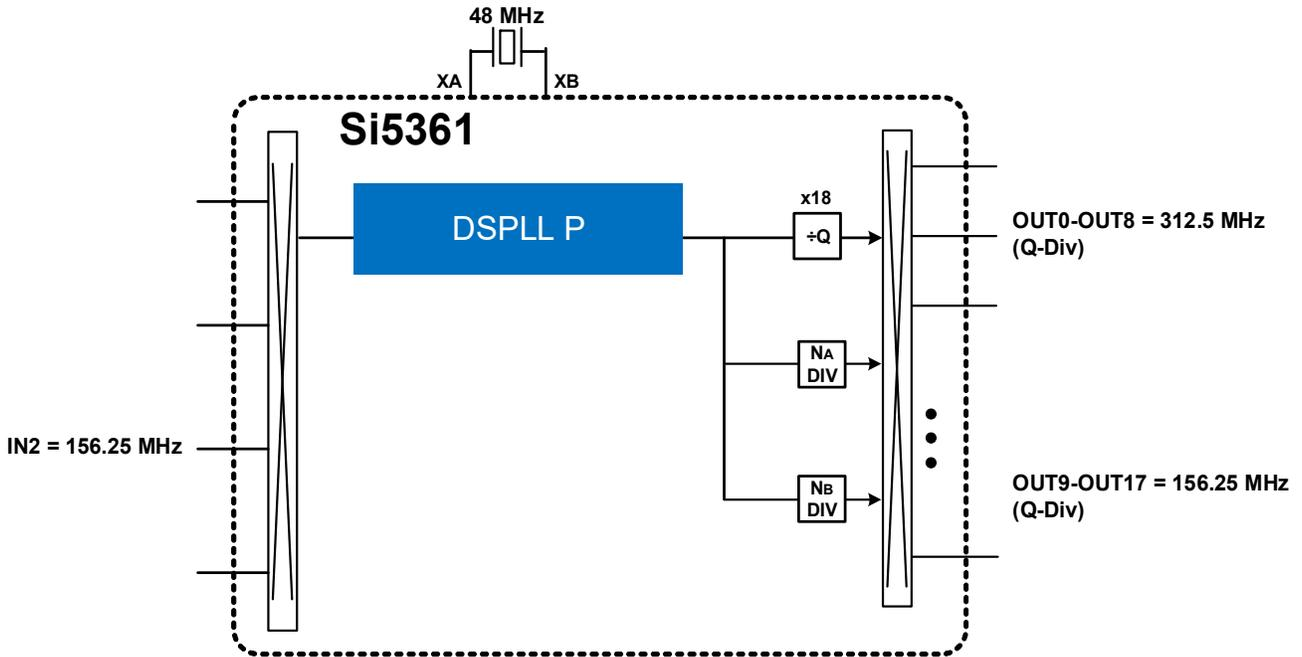
Figure 8. Si5361 Typical Operating Circuit
