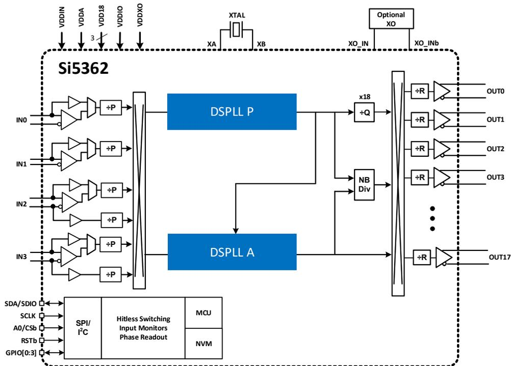
Figure 2. Si5362 Simplified Block Diagram (2x DSPLL + 1x MultiSynth)
