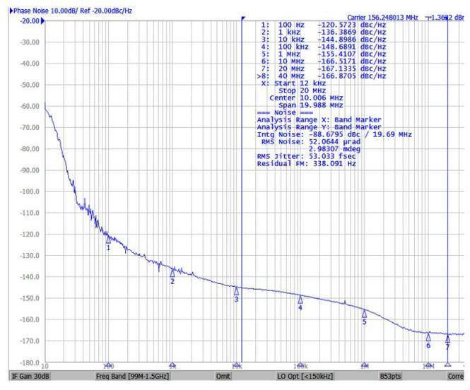
Figure 12. 53 fs RMS Jitter for SyncE 156.25 MHz
