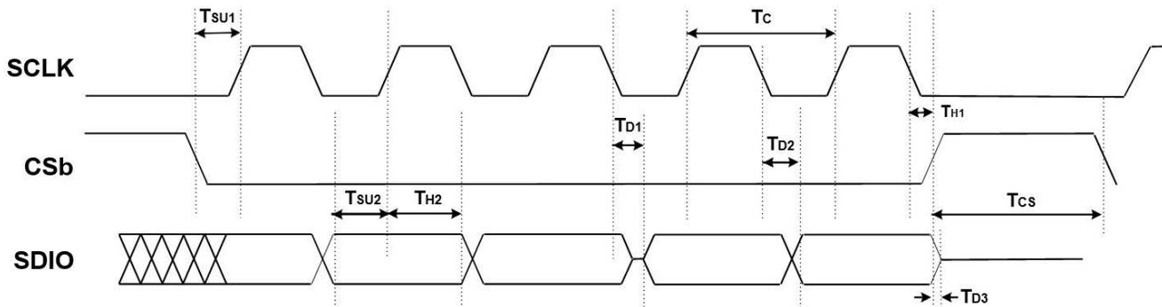
**Figure 9. 3-Wire SPI Serial Interface Timing**
