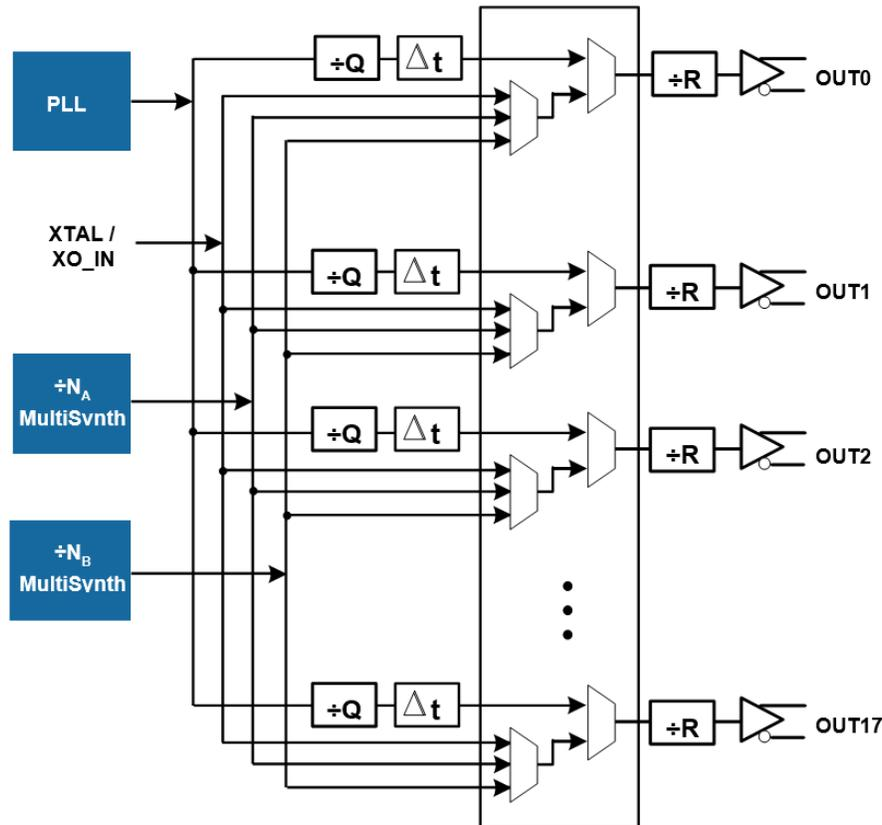
Figure 5. Output Structure
