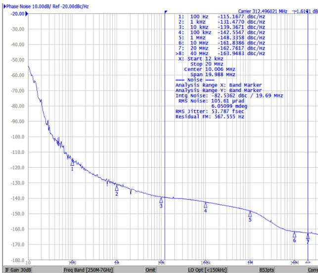
Figure 11. 53.7 fs RMS Jitter for SyncE 312.5 MHz
