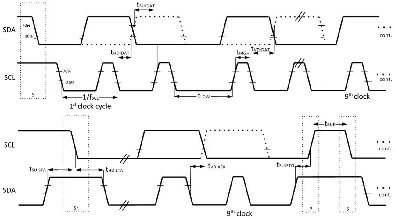
Figure 7. I<sup>2</sup>C Serial Port Timing Standard and Fast Modes
