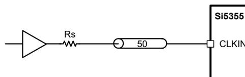
Figure 3. Interfacing CMOS Reference Clocks to the Si5355
