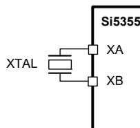
Figure 2. Connecting an XTAL to the Si5355
