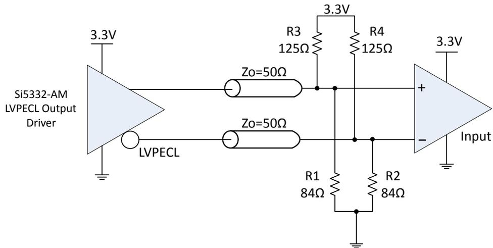
**Figure 3.8. 3.3 V LVPECL Output Termination, Option 2**
