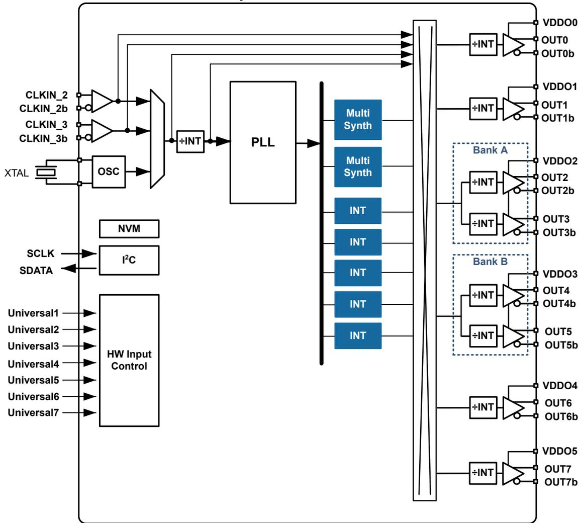
Figure 3.2. Block Diagram for 8-Output Si5332 in 40-QFN
