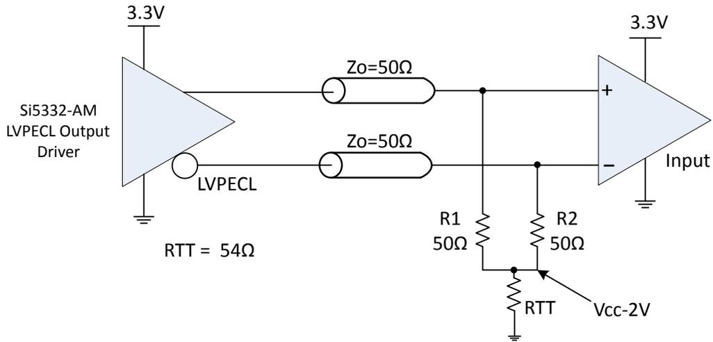
**Figure 3.7. 3.3 V LVPECL Output Termination, Option 1**
