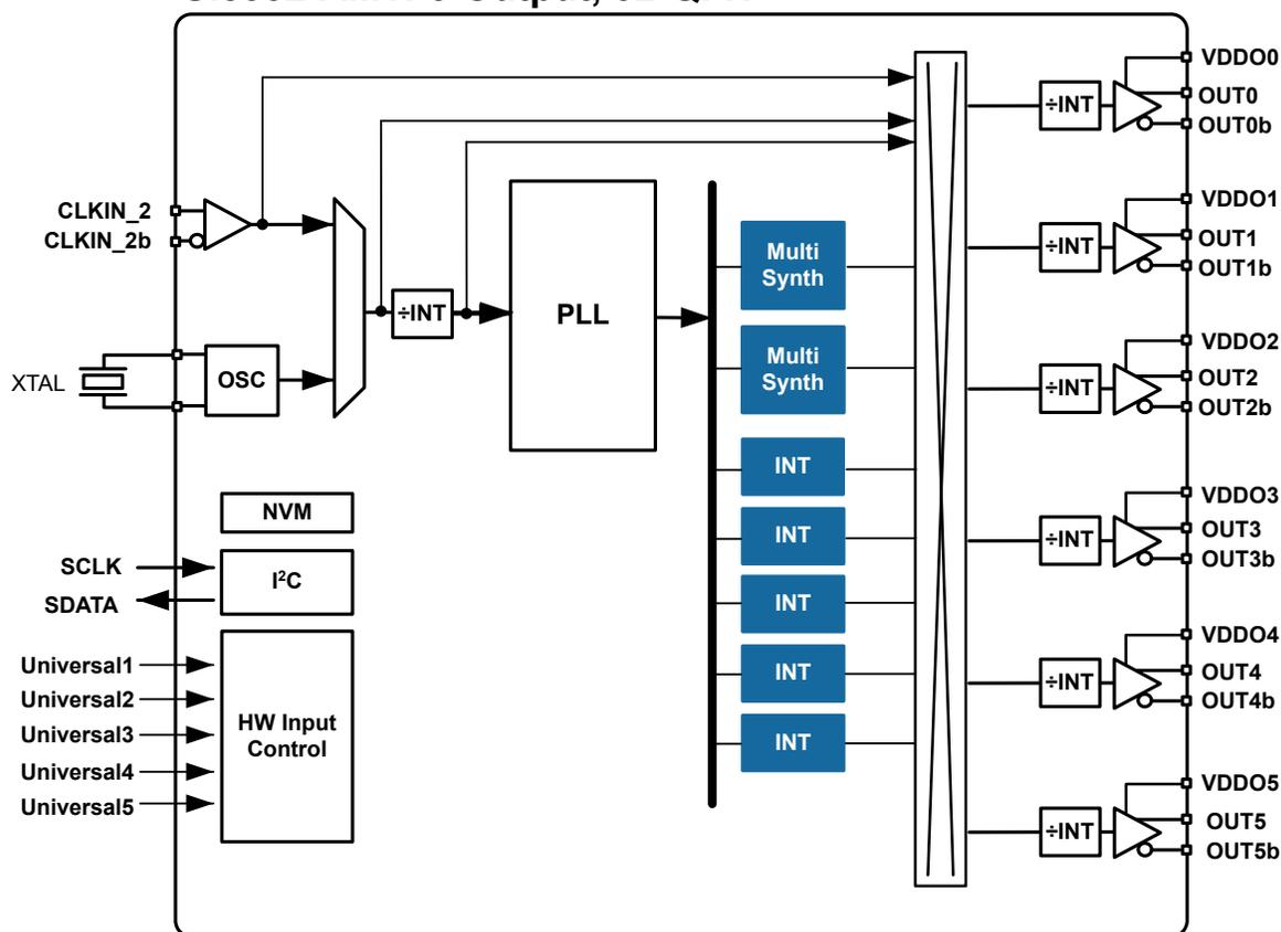
**Figure 3.3. Block Diagram for 6-Output Si5332 in 32-QFN**
