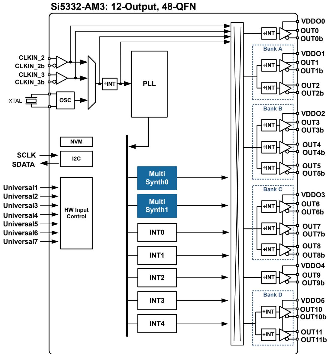
Figure 3.1. Block Diagram for 12-Output Si5332 in 48-QFN
