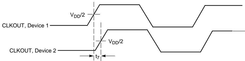
Figure 6. Device-Device Skew
