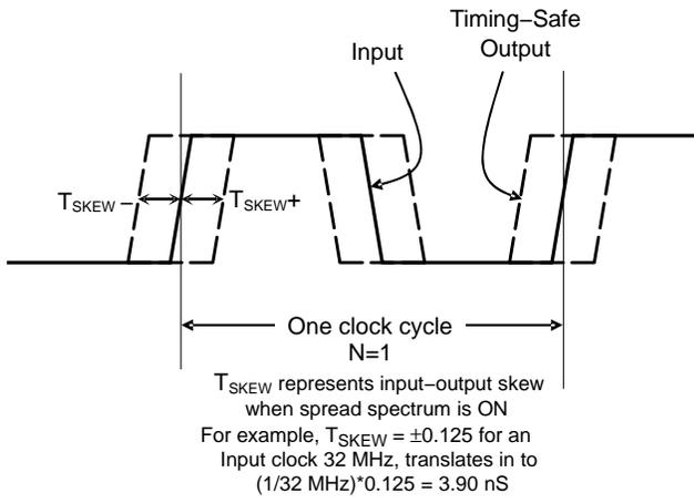
Figure 7. Input-Output Skew
