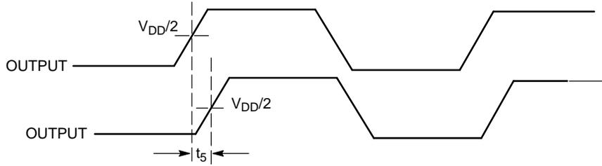
Figure 4. Output-Output Skew
