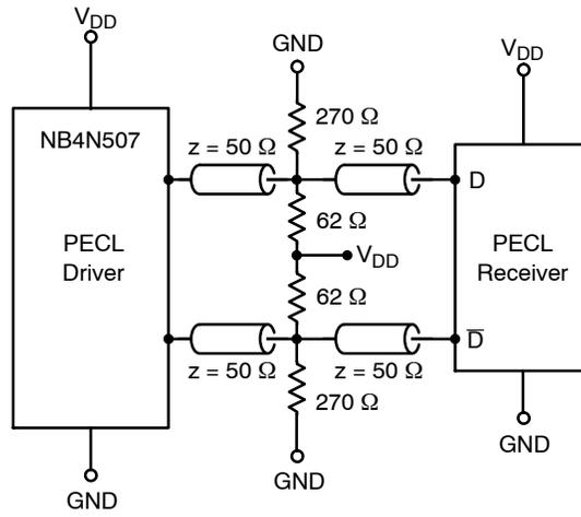
Figure 5. Evaluation Test Load for the NB4N507A
