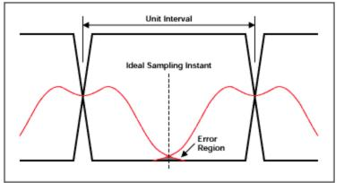
Figure 2. Ideal eye diagram with data transition time probability histograms.
