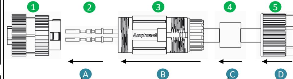
**A** Audio and handling feedback while assembling, and pull cable to make sure.
