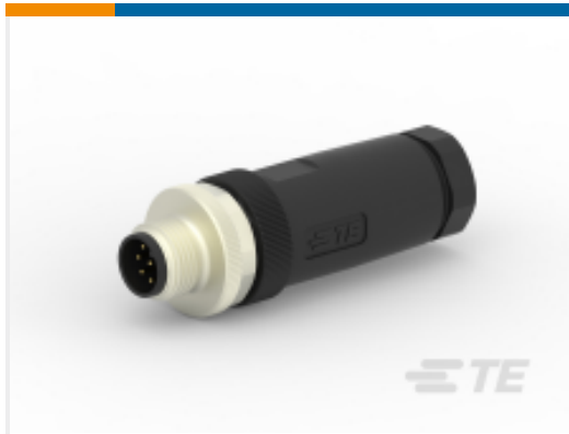
TE Part #T4111002081-000 M12, MALE, STRAIGHT, A CODE, 8P, PG9, GOLD
