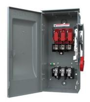
Siemens Low Voltage Circuit Protection Heavy Duty Safety Switch. 3-Pole 3-Wire Non-Fused in a type 1 enclosure (indoor). Rated 600VAC (60A). Special features: photovoltaic rated, positive ground, 10000 AIC disconnect.
