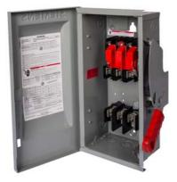
Siemens Low Voltage Circuit Protection Heavy Duty Safety Switches. Type: ENCLOSED, SAFETY SWITCH Std: CSA V. Rating: 600V A. Rating: 200A Wattage: 4W No. Of Poles: 3P F. Rating: 60Hz Action: SINGLE THROW Material: STEEL Enclosure: TYPE 1. 2-3 point mounting holes. O. Cycles: 8000 O. Temperature: (-20F-120F) AMBIENT TEMPERATURE Environmental Conditions: INDOOR
