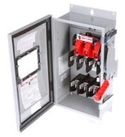
Siemens Low Voltage Circuit Protection Heavy Duty Safety Switches. Type: ENCLOSED, SAFETY SWITCH Std: CSA V. Rating: 600V A. Rating: 200A Wattage: 3W No. Of Poles: 3P F. Rating: 60Hz Action: SINGLE THROW Material: 304SS Enclosure: TYPE 12. 2-3 point mounting holes. Insulation: YES O. Cycles: 8000 O. Temperature: (-20F-120F) AMBIENT TEMPERATURE Environmental Conditions: INDUSTRIAL
