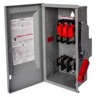
Siemens Low Voltage Circuit Protection Heavy Duty Safety Switches. Type: ENCLOSED, SAFETY SWITCH Std: CSA V. Rating: 600V A. Rating: 100A Wattage: 3W No. Of Poles: 3P F. Rating: 60Hz Action: SINGLE THROW Material: 304SS Enclosure: TYPE 3R. 2-3 point mounting holes. O. Cycles: 10000 O. Temperature: (-20F-120F) AMBIENT TEMPERATURE Environmental Conditions: OUTDOOR
