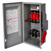
Siemens Low Voltage Circuit Protection Heavy Duty Safety Switches. Type: ENCLOSED, SAFETY SWITCH Std: CSA V. Rating: 600V A. Rating: 100A Wattage: 4W No. Of Poles: 3P F. Rating: 60Hz Action: SINGLE THROW Material: 304SS Enclosure: TYPE 3R. 2-3 point mounting holes. O. Cycles: 10000 O. Temperature: (-20F-120F) AMBIENT TEMPERATURE Environmental Conditions: OUTDOOR
