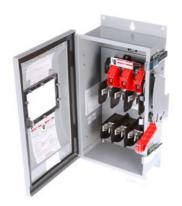
Siemens Low Voltage Circuit Protection Heavy Duty Safety Switches. Type: ENCLOSED, SAFETY SWITCH Std: CSA V. Rating: 600V A. Rating: 100A Wattage: 3W No. Of Poles: 3P F. Rating: 60Hz Action: SINGLE THROW Material: 304SS Enclosure: TYPE 12. 2-3 point mounting holes. Insulation: YES O. Cycles: 10000 O. Temperature: (-20F-120F) AMBIENT TEMPERATURE Environmental Conditions: INDUSTRIAL
