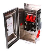
Siemens Low Voltage Circuit Protection Heavy Duty Safety Switches. Type: ENCLOSED, SAFETY SWITCH Std: CSA V. Rating: 240V A. Rating: 30 A Wattage: 3W No. Of Poles: 3P F. Rating: 60Hz Action: SINGLE THROW Material: SS Enclosure: TYPE 4X. 2-3 point mounting holes. Insulation: YES O. Cycles: 10000 O. Temperature: (-20F-120F) AMBIENT TEMPERATURE Environmental Conditions: INDUSTRIAL CORROSIVE RESISTANCE
