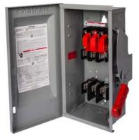
Siemens Low Voltage Circuit Protection Heavy Duty Safety Switches. Type: ENCLOSED, SAFETY SWITCH Std: CSA V. Rating: 240V A. Rating: 200A Wattage: 3W No. Of Poles: 2P F. Rating: 60Hz Action: SINGLE THROW Material: STEEL Enclosure: TYPE 1. 2-3 point mounting holes. O. Cycles: 8000 O. Temperature: (-20F-120F) AMBIENT TEMPERATURE Environmental Conditions: INDOOR
