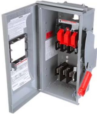
Siemens Low Voltage Circuit Protection Heavy Duty Safety Switches. Type: ENCLOSED, SAFETY SWITCH Std: UL V. Rating: 600V A. Rating: 60A Wattage: 3W No. Of Poles: 3P F. Rating: 60Hz Action: SINGLE THROW Material: 304SS Enclosure: TYPE 3R. 2-3 point mounting holes. O. Cycles: 10000 O. Temperature: (-20F-120F) AMBIENT TEMPERATURE Environmental Conditions: OUTDOOR
