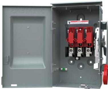
Siemens Low Voltage Circuit Protection Heavy Duty Safety Switches. Type: ENCLOSED, SAFETY SWITCH Std: UL V. Rating: 600VDC A. Rating: 60A Wattage: 3W No. Of Poles: 3P F. Rating: 60Hz Action: SINGLE THROW Material: 304SS Enclosure: TYPE 3R. 2-3 point mounting holes. O. Cycles: 10000 O. Temperature: (-20F-120F) AMBIENT TEMPERATURE Environmental Conditions: OUTDOOR
