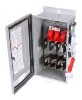
Siemens Low Voltage Circuit Protection Heavy Duty Safety Switches. Type: ENCLOSED, SAFETY SWITCH Std: UL V. Rating: 240V A. Rating: 100A Wattage: 3W No. Of Poles: 3P F. Rating: 60Hz Action: SINGLE THROW Material: 304SS Enclosure: TYPE 12. 2-3 point mounting holes. Insulation: YES O. Cycles: 10000 O. Temperature: (-20F-120F) AMBIENT TEMPERATURE Environmental Conditions: INDUSTRIAL
